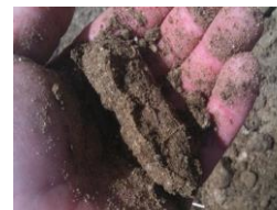
Soil sample with high sand content. The sample is unable to form a ribbon.
