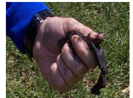
Soil sample with high clay content. The sample is able to ribbon 2 inches.
